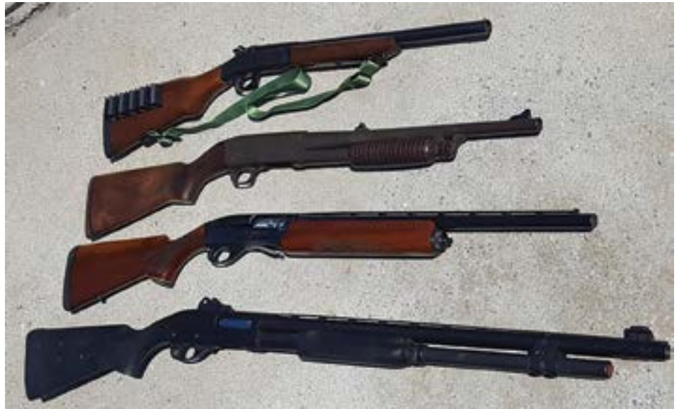
"Old School" Shotguns. (top to bottom) Harrinton & Richardson "Topper" Single-shot 12 gauge, 18.15" bbl. and 5-round stock carrier. Ithaca Model 37, Police surplus "Deerslayer", pump action 12 gauge. Remington 1100 Semi-automatic, with Speedfeed magazine gate, 21" bbl. fitted for RemChokes. Remington 870 "Wingmaster", factory 26" bbl. w/interchangeable chokes, +5-round magazine tube, X/S barrel band front sight, and VangComp rear sight.
